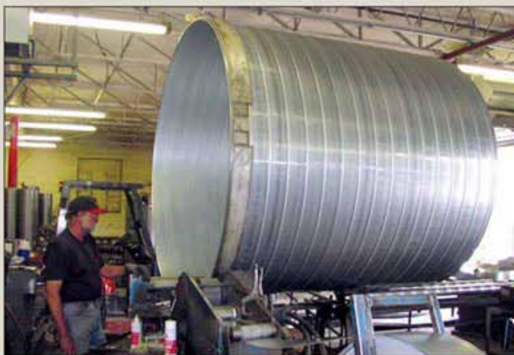
Making some of the 78-inch-diameter galvanized ductwork the Fort Worth, Texas, Cabela's store would use.
