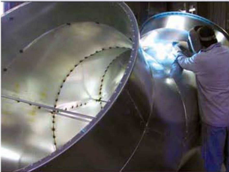
An unidentified Spiral Pipe of Texas employee welds a 58-inch-diameter, 90-degree elbow for use in Cabela's.
